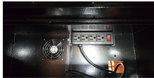
Left: Interior overview showing FM transmitter (left), DeerTV cooling fan (center), and power strip (right). Right: Close-up of 4-outlet power strip and internal cooling fan.
