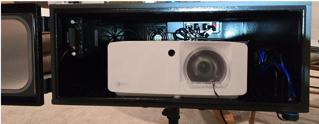
Fully loaded interior: Optoma GT2100HDR projector seated in main bay with all electronics installed above.
