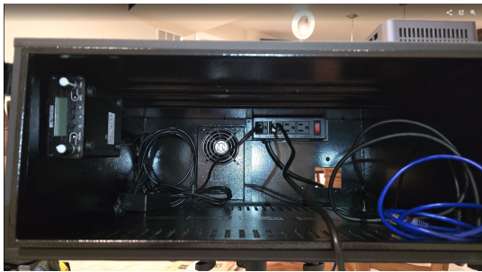
Left: Interior overview showing FM transmitter (left), DeerTV cooling fan (center), and power strip (right). Right: Close-up of 4-outlet power strip and internal cooling fan.
