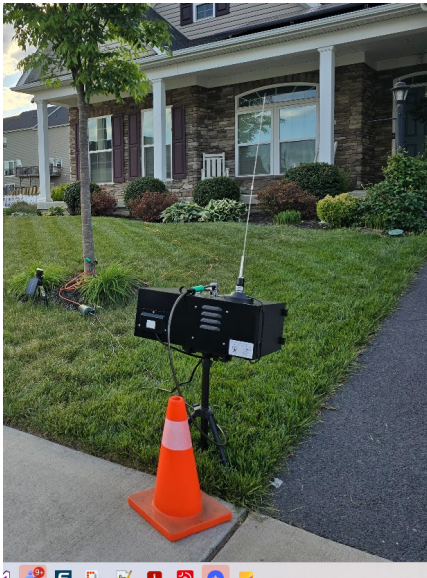
Left: Fully deployed rig on front lawn with FM antenna extended and security cone placed. Right: Trampoline anchor stake driven through tripod leg foot for wind resistance.
