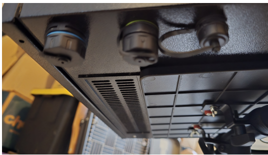
Left: Bottom edge showing installed Ethernet (blue), USB-A (green), and USB-C connectors. Right: Right side panel with FM antenna feedthrough installed solo.
